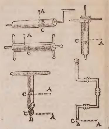
All which are but severall kinds of this third Mechanicall faculty. In which the points ABC, doe represent the places of the power, the fulciment, and the weight. The power being in the same proportion unto the weight, as B C is unto B A.
